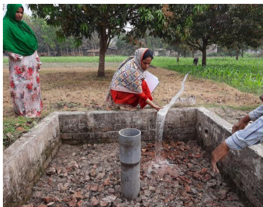
Fig. 1. Infiltration rate measurement at ASR trial setup, Paba, Rajshahi
