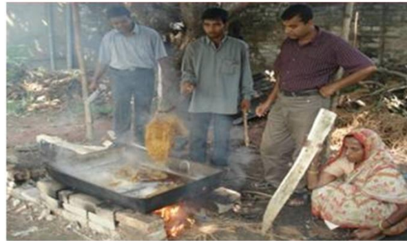
Fig. 1: Heating process of coir fibre and yarn in hydrogen peroxide bleaching solution.
