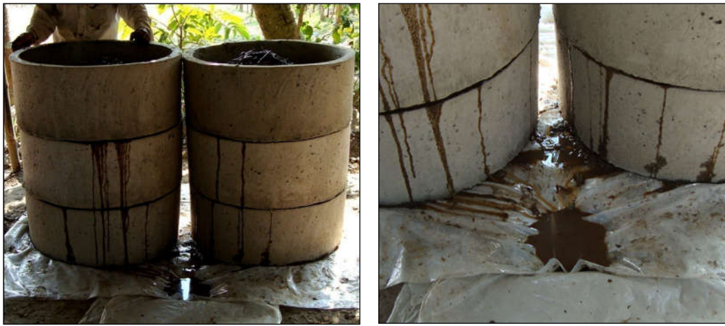
Fig. 5. After loading raw materials in composting device (left), leachate (right) coming out
