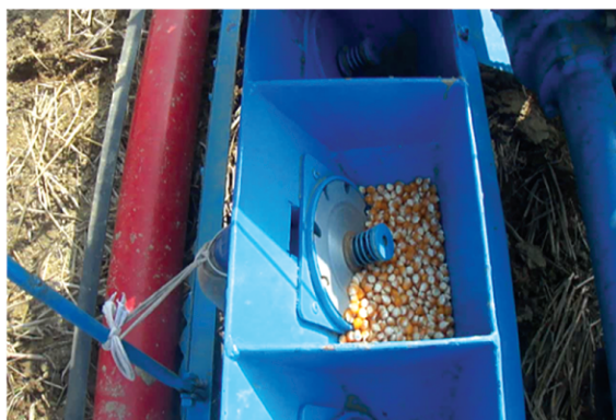
Seed pot and seed plate of the BARI Seeder machine
