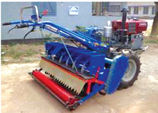
The BARI seeder machine hitched to a power tiller
